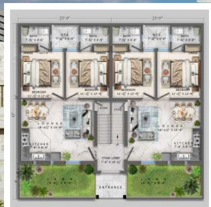
GROUND FLOOR PLAN Covered Area = 816 sft (Per Town House)
